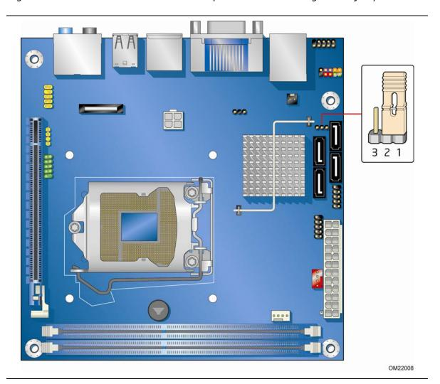
Figure 24. Location of the BIOS Configuration Jumper Block
